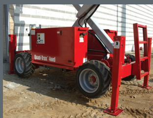
Operators just "flick a switch" to activate outriggers for slightly off-level surfaces.
